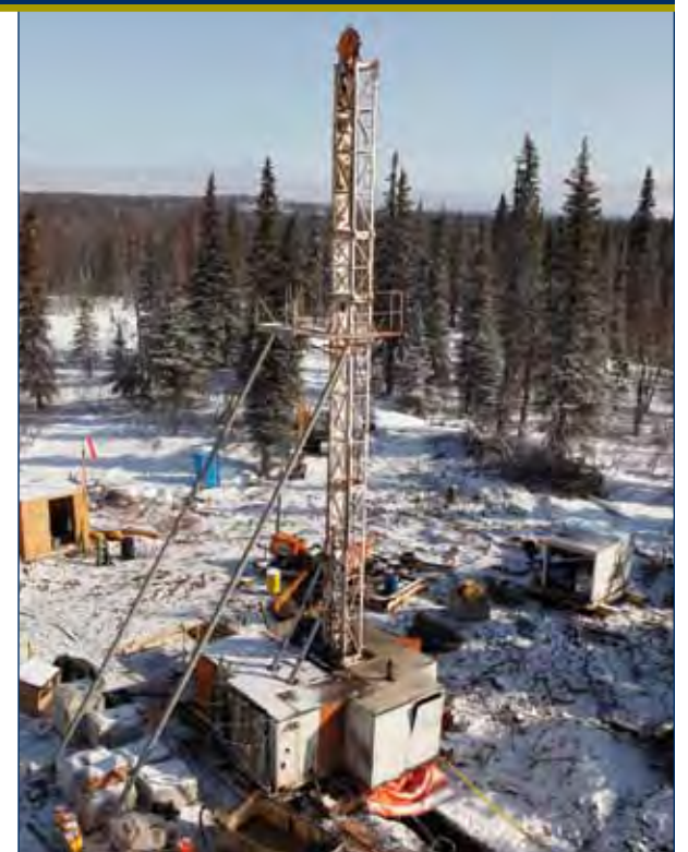
The test drilling conducted for the project this last spring confirmed the existence of a large coal resource appropriate for underground coal gasification development.
