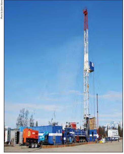
A work-over rig NordAq is using to explore CIRI's subsurface resource.
